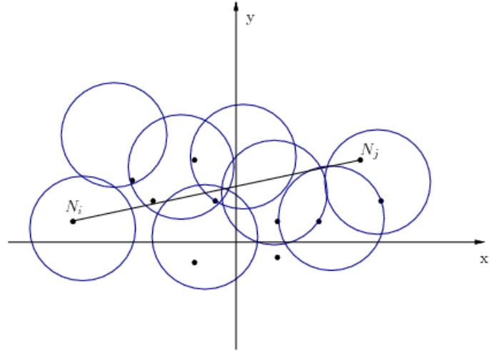
Fig. 1. An illustration of a non-uniform damage process. Dots represent the sensor nodes and circles are the damage circles with their centers being the damage center locations.
